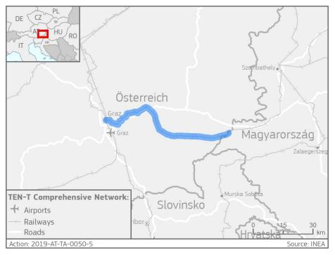
The railway line connecting the second biggest city of Austria, Graz, with Györ in Hungary is currently not electrified between Graz and Szentgotthárd.
