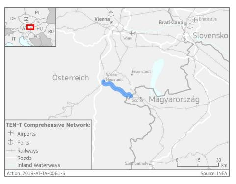
The railway line from Wiener Neustadt to Sopron is a non-electrified, single track railway line with a length of 33.7 km.
