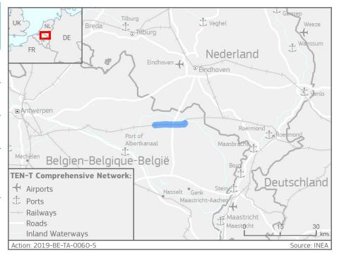
The Action is located on the comprehensive network and concerns a study to construct a second electrified track of approximately 13,3 km between Balen-Werkplaatsen and Neerpelt (part of the global project to construct a double electrified track on the 3RX-Route as a competitive alternative route between the North Sea ports and the Rhein Ruhr Area).
